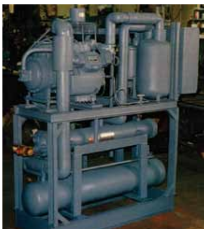
Custom designed and built blast freeze refrigeration unit for a fishing vessel.
