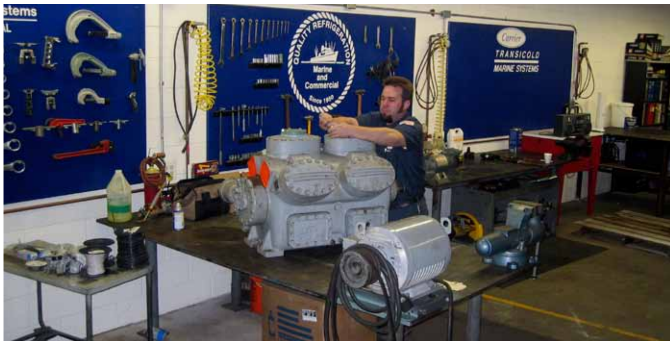
Quality Refrigeration's Compressor Rebuilding Station, in the company's San Diego location. Shown is Technician Mike Scott.
